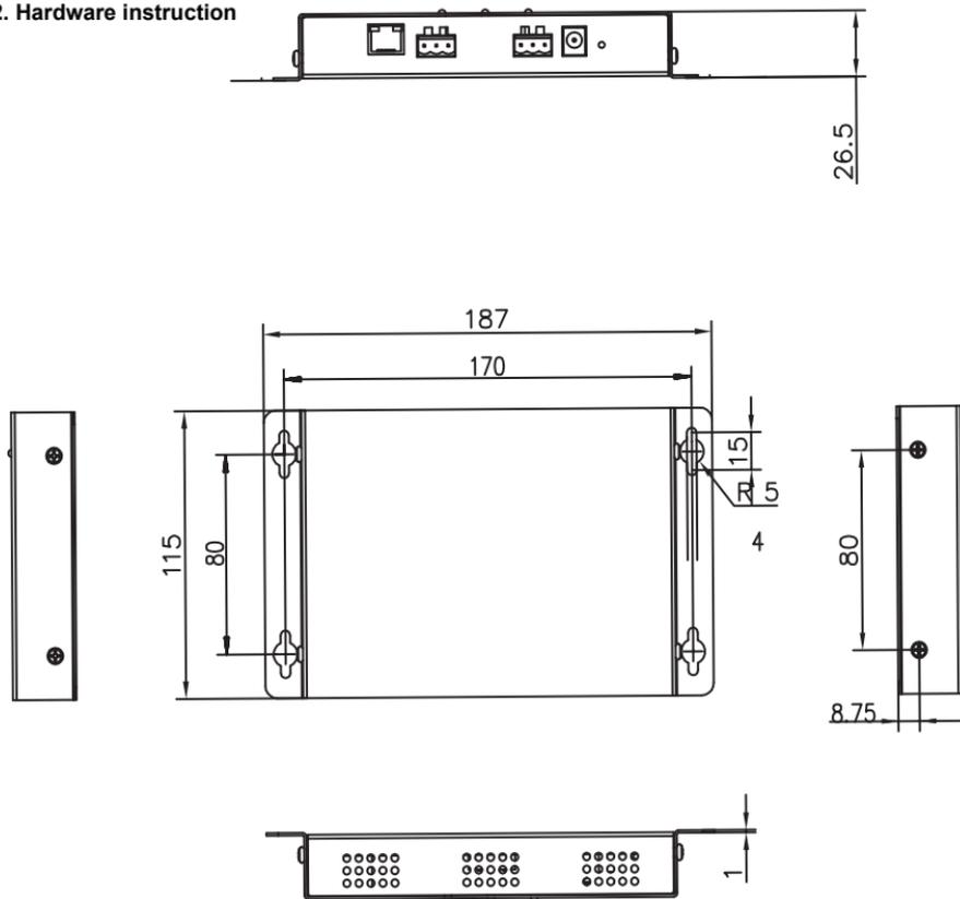
Fig.3.1 Structure dimension drawing
